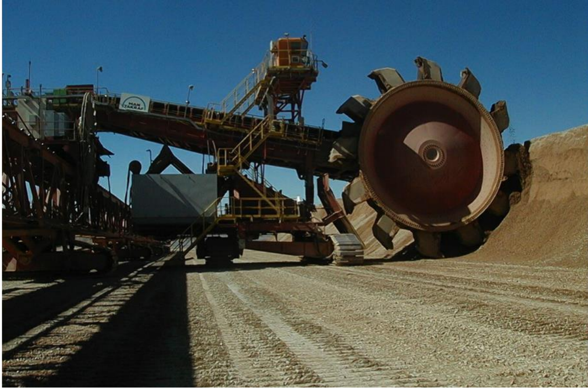
Figure 18: Race-track system with bucket wheel excavator in northern Chile
