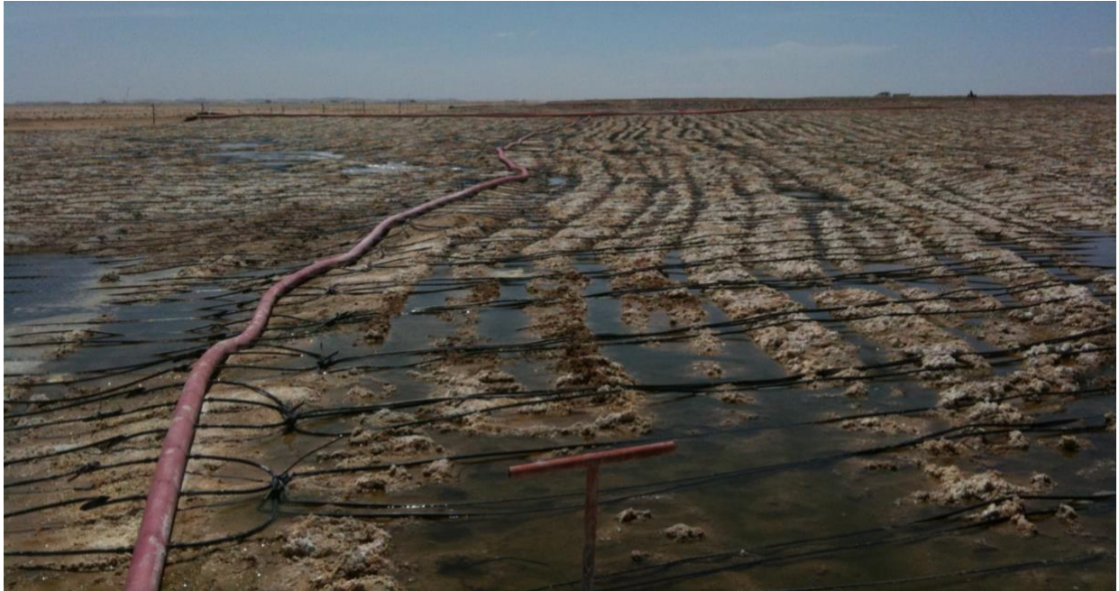
Figure 12: Chemical and biological fouling on a carbonate uranium HLF in Namibia
