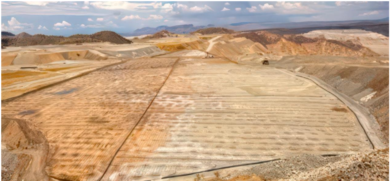
Figure 3: Copper sulfide dump bioleaching at the Morenci mine, Arizona, USA
