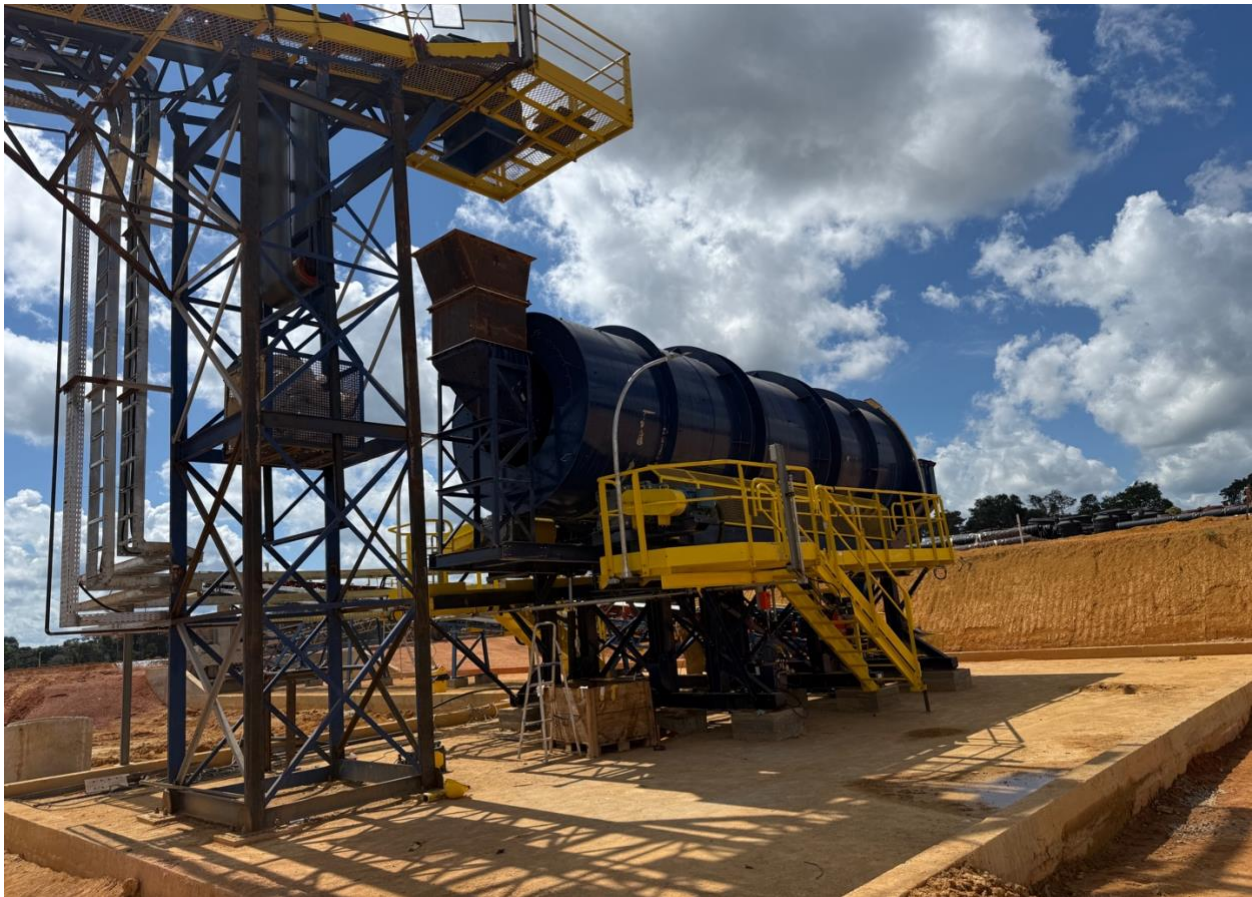
Figure 24: Agglomeration drum for gold ore at the Cuiú Cuiú gold mine in northern Brazil
