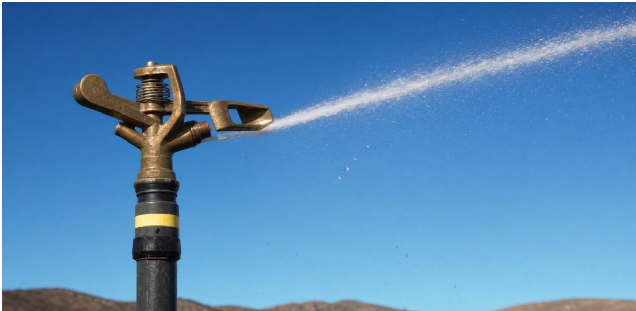
Figure 26: Impact sprinklers used in some dump leaching to increase evaporation
