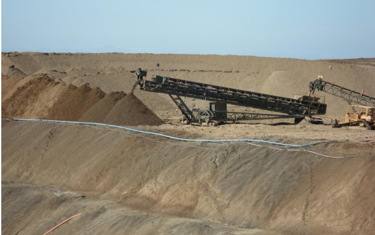
Figure 15: Retreat stacking with a radial stacker system in Central America
