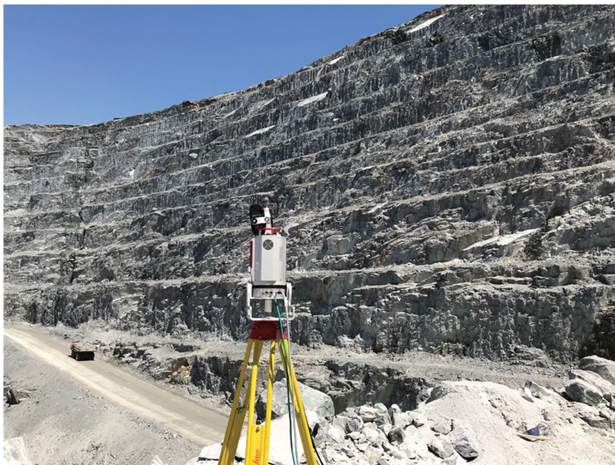
Figure 2 Laser scanner survey done on a wall of an open pit mine selected as test site
