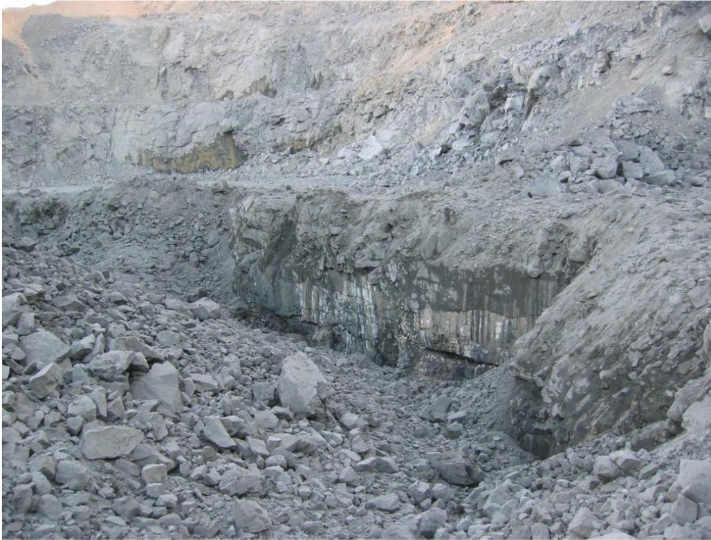
**Figure 9** – Sheet Joint with Groundwater Flowing in 120 Level Sequeirinho Pit. schists.
