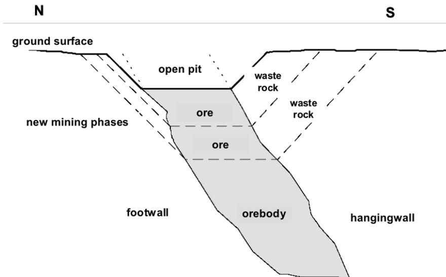
**Figure 4** - Schematic of Sequeirinho Pit Mining in Phases.
