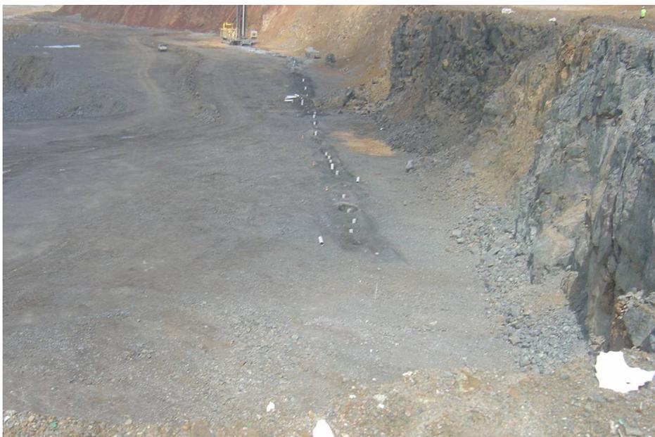
**Figure 20** - Sossego Pit Phase 2. Note the jointing pattern and weathering variation of the rock mass. Vertical 311mm blast holes were used for the controlled blast.
