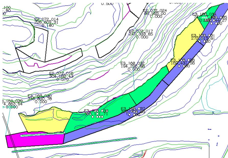
**Figure 14** - Typical Planning of Blasts at Sossego Mine. The Blue Space indicates the region where trim blasting was used (typically 25m from the toe). The other areas are production blasts.
