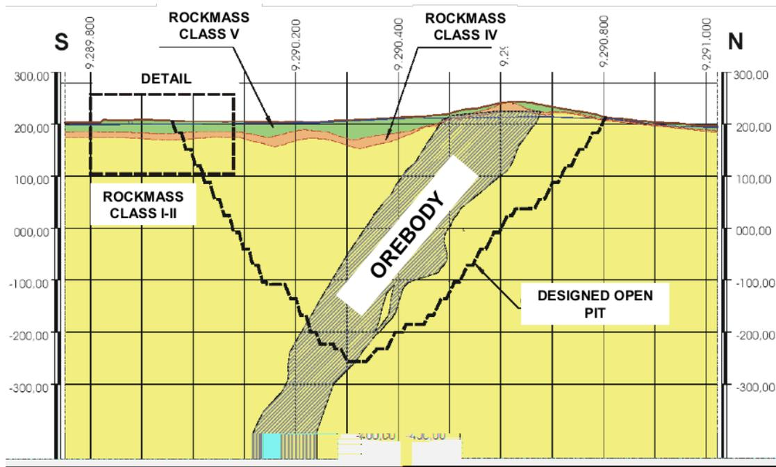
**Figure 8a** - Sequeirinho Pit Geomechanical Cross-Section.
