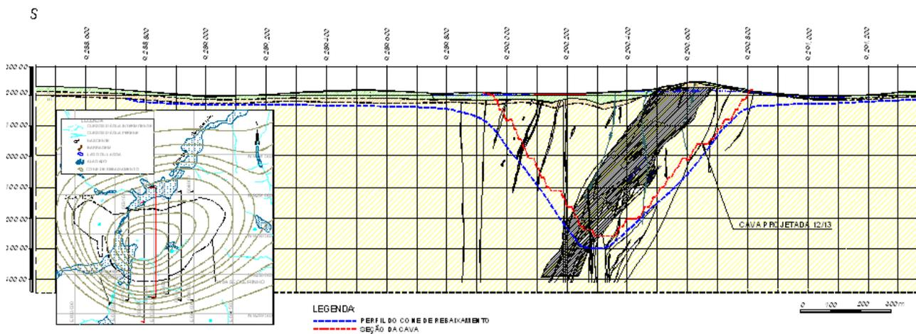
**Figure 10** - Water Table at Sequeirinho Pit after 13 years of Mining Operation.
