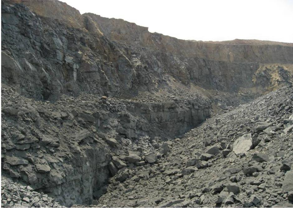
**Figure 11** - Blast Damage in Sossego Pit
