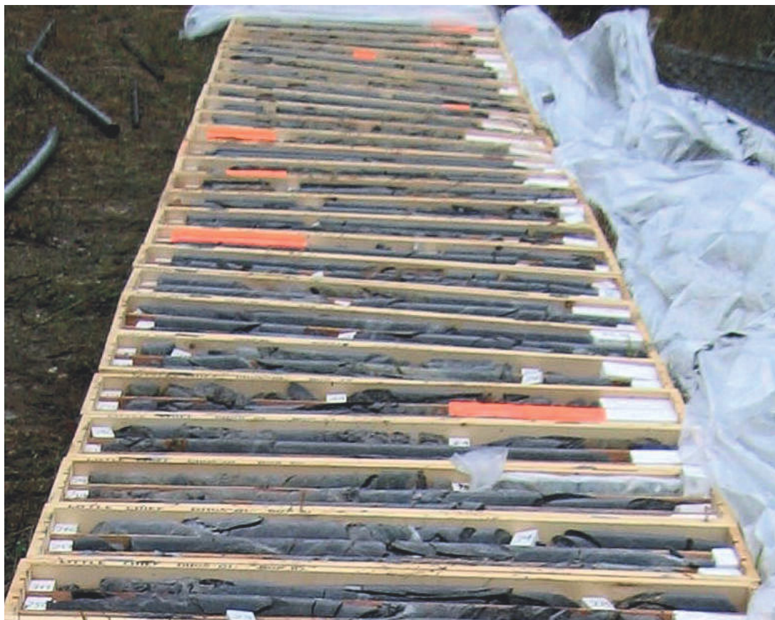
Figure 12: Core loss zones marked by red coloured lengths of PVC (source: D Martin)
