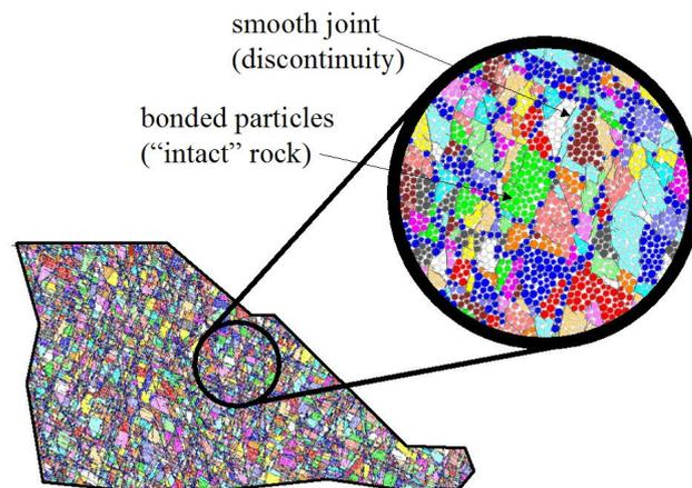
Fig. 4. A two-dimensional SRM model used to study slope failure mechanisms.
