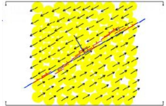
Fig. 2. By using the smooth joint contact model to reorient all contacts lying along the macroscopic joint plane, sliding along a smooth planar feature can be more accurately modeled.
