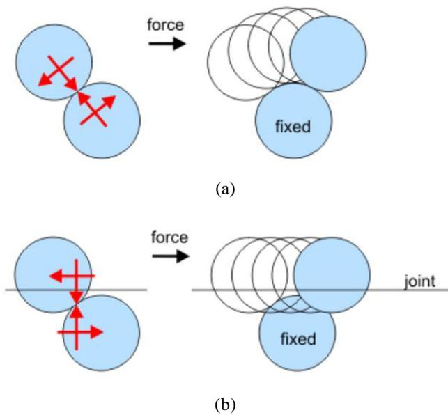
Fig. 1. Graphical representation of how the smooth joint contact model can be used to realign the default contact orientation (a) to one that honors a macroscopic joint orientation (b).
