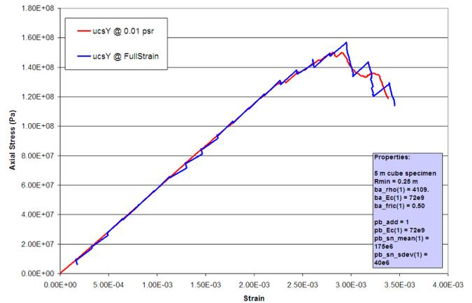
Fig. 3. A comparison of stress-strain behavior derived from a normal platen-based test on an SRM material versus one in which full strain logic is employed.
