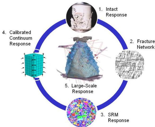
Fig. 5. Characterization of the large-scale response of a rock mass using the Synthetic Rock Mass approach combined with continuum modelling.
